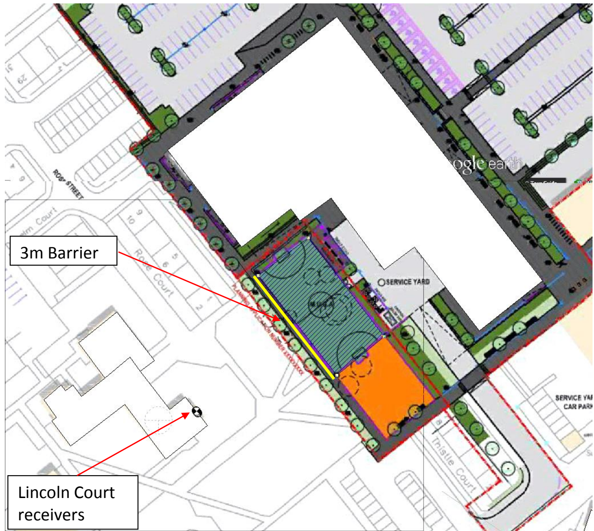
Figure 2: Plan view of CadnaA model illustrating receiver position, barrier shown as yellow line
